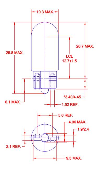
\*TO BE MEASURED ON LONGEST SIDE ONLY WITH THE WIRE IN INTIMATE CONTACT WITH THE BOTTOM OF THE GLASS WEDGE.
