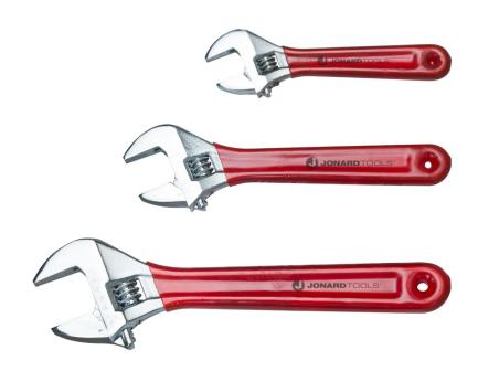
Jonard's adjustable wrenches are made of chrome vanadium steel with a chrome plated finish. They are forged and heat treated for maximum strength. Handles are covered with a red vinyl grip for user comfort. The knurled worm gear is precision formed and the operation is smooth and trouble free. For acurate and faster adjustments use the metric or English scales on either side of the jaws. With extra wide jaws, a smaller wrench works on bigger jobs. Great for tight spaces.
