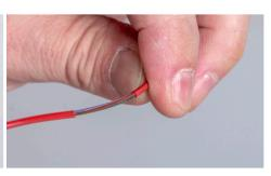
The Jonard Tools **BTR-6** Buffer Tube Ring tool provides quick access to fibers inside buffer tubes up to 6mm in diameter and will work with buffer tubes with wall thicknesses up to 1mm. The tool is light and durable with a hardened steel blade for long life. Includes hole for tethering.
