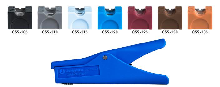
The CSS Series tools are coaxial cable strippers specifically designed to strip a stub end of a coax cable in a wall outlet box, which eliminates the need to run new cable, saving time and money. Each strips RG-59 and RG-6 cables to specific braid and center conductor lengths shown in chart below. The built-in strip stop insures the strip lengths are consistent. VELCRO® strip on bottom of tool is used to fold back braid on cable after being stripped.
