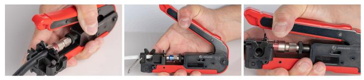
Using specially designed jaws to hold connectors in place while compressing, this **PATENTED** CTF-360 is designed to hold and compress connectors requiring a full 360 degree support. Perfect tool for short F connectors for RG59/6 cables and F connectors for RG7/11 cables. This tool also features the following:
