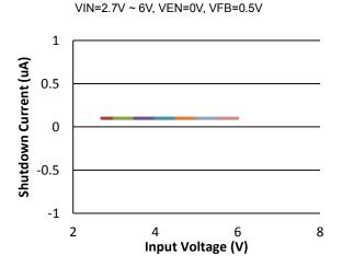
Shutdown Current Vs. Input Voltage
