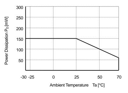
**Power Dissipation - Ambient Temperature Characteristic**
