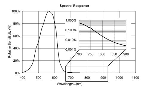
Resistance to optical noise of AC lamps
