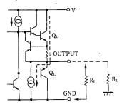
NJM2902, in its static state (No in and output condition) when design, Q<sub>U</sub> being biassed by constant current (breake down beam) yet, Q<sub>L</sub> stays OFF.
