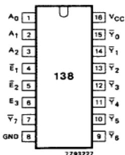
Fig.1 Pin configuration.
