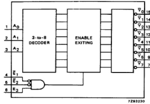
Fig.4 Functional diagram.
