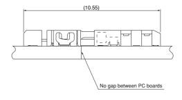
Note: 1. The above figure is the figure viewed from the connector mounting side.
