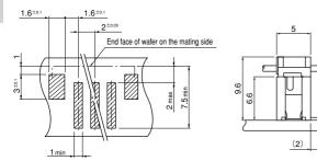
Note: 1. The above figure is the figure viewed from the connector mounting side. 2. Tolerances are non-cumulative: ±0.05 mm for all centers
