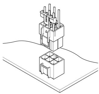
This VL connector is 6.2 mm pitch wire-towire and wire-to-board connector, designed for large current. Secondary retainer, which prevents from insufficient insertion of contact and coming off contact, may use and large current circuit can be connected certainly and safety.
