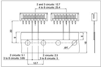
Note: Conforms to JIC C 0806 of "Tape packaging of components with unidirectional leads on continuous tapes".
