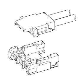
Considering about the luminescence property of LED package, this LEN connector is designed as low profile type connector for LED lighting. In consideration of connector mating operation to the LED mounting PCB that is integrated in the equipment, side-feed mechanism that provides to enable mating the connector from above is adopted, and secure lock that considered handling and mechanism for preventing wrong insertion are provided.
