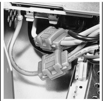
The CL is a low-voltage, insulation displacement connector that can be applied using simple tools.
