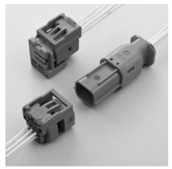
Compliant with the ISO 19689, 0.64 mm individual waterproof, 6 pole wire to wire connection connector. The retainer is a pre-set type for both female and male housing.
