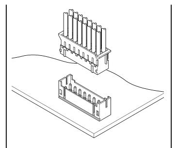
This is a 2.0 mm pitch, crimp style, dual-row, wire-to-board connector. It is designed to meet the demand for high-density and low-profile connection.
