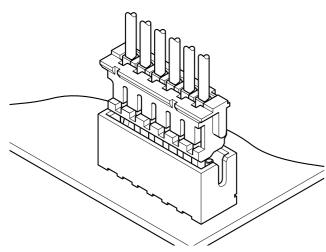
The ZH connector is very small with a mounting height of 5.6mm and a thickness of only 3.5mm. Contact retention lances on the housing make insertion easier, while the dimple at the center of the contact ensures reliable contact with the post.
