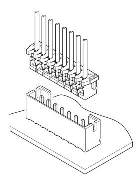
Multi-harness of CK connector (2.0mm) and CZ connector (1.5mm) combination has been realized. The in-line type IDC features low profile design with 6.9mm mounting height and 4.8mm thickness (top entry type).
