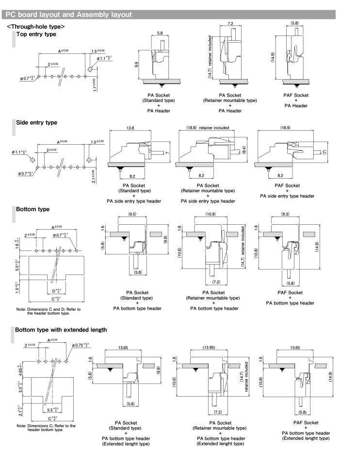
Note: 1. The above figure is the figure viewed from the connector mounting side.
