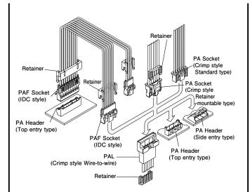
Based upon wire-to-board crimp style PA connectors, the PA series family of connector have been expanded to meet the requirement of complex wire harness of 2.0 mm pitch connectors with secure locking mechanism thanks to the additional line up of wire-to-board IDC style PAF connectors and wire-to-wire crimp style PAL connectors.
