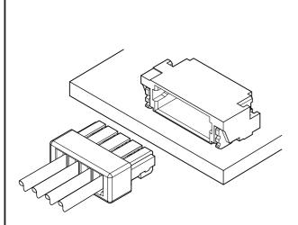
This SUH connector is developed for crimping type SUR connector that has been designed for 0.8 mm pitch wire-toboard insulation displacement connector. This connector adopted the first crimping method in a minimum 0.8 mm pitch of the wire-to-board type connector. Housing lance method provides the good workability and a constriction contact method provides the excellent contact reliability.
