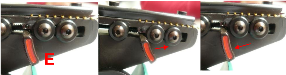
Push in until the locking lever (E) engages with the strip lock and the feed can be effected by yellow feed lever (G, see picture 7).
