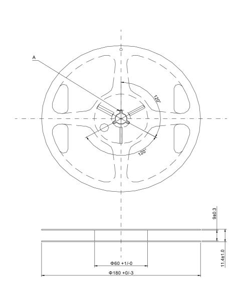
Material:Polystyrene (Conductivity) unit:mm
