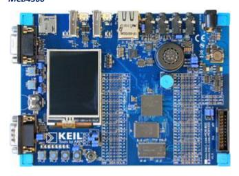
The Keil MCB4300 Evaluation Board enables you to create and test working programs based on the NXP LPC4300 family of ARM Cortex<sup>™</sup>-M4 processor-based devices.
