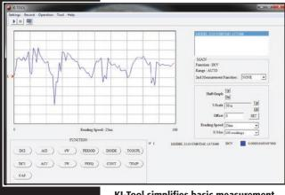
KI-Tool simplifies basic measurement applications through every setup and graphical data representation. including graphical, statistical, and trend charting. A version supporting Microsoft Word is also included for direct data import into reports.
