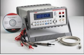
All accessories, such as start-up software, USB cable, power cable, and safety test leads, are included with the Model 2110.
