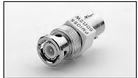
Model 7755 50Ω Feed-Through Terminator: BNC-to-BNC adapter for terminating RG58 cable in its characteristic impedance. VSWR <1.1, DC-250MHz.
