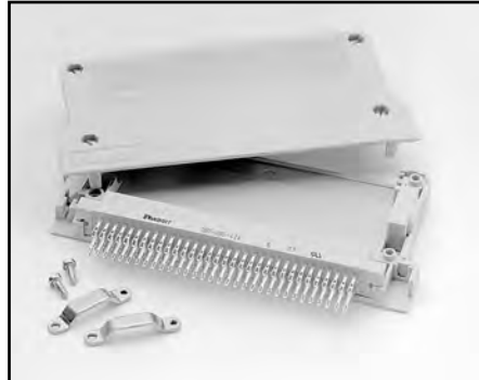
Model 7011-KIT-R: 96-pin female DIN connector with solder eyelets and strain relief. This kit can be used for assembly of custom cables to connect with the connectors on the 7011-C, 7012-C, 7013-C, 7015-C, and 7018-C switch cards. Also connects with the 7011-MTR bulk-head mount male connector.
