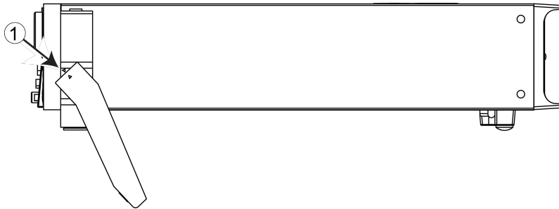
Figure 7: Line up arrows on handle
