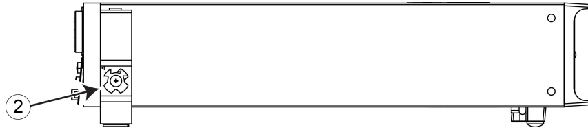
Figure 9: Remove mounting ears
