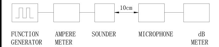
In the measuring test, buzzer is placed as follows:
