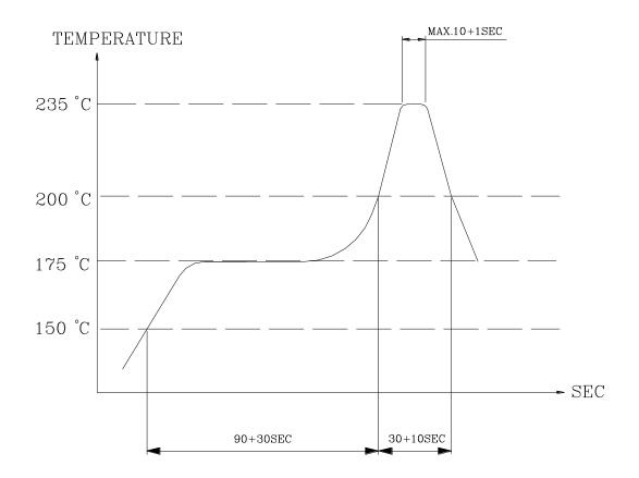
Heat resistant line (Used when heat resistant reliablity test is performed)
