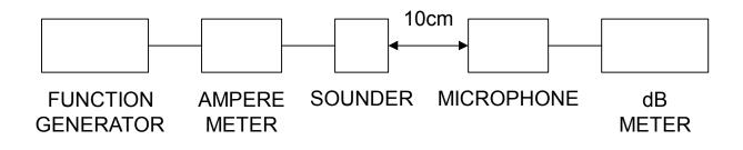
In the measuring test, buzzers is placed as follows:
