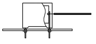
Temperature monitored inside the capacitor.
