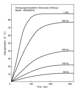
Figure 9 - Heat Generation vs. Drive Frequency - 2
