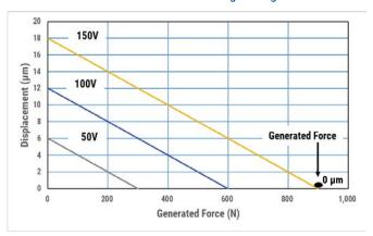
Figure 4 - Generated Force vs. Displacement - 2
