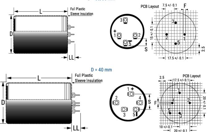
Connections: Hole 1 represents +ve. Hole 5 Represents -ve. Terminals 2,3, and 4 may be at negative terminal potential due to the presence of electrolyte. They are intended for mechanical connections only. It is recommended that they are soldered to the printed cicuit board. Additional dummy pins are provided for stability. Note that the case and dummy pins may be at negavtive terminal potential
