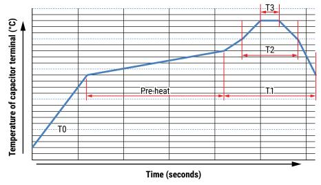
Vapor heat transfer systems are not recommended. The system should be thermal, such as infra-red radiation or hot blast Observe the soldering conditions as shown below.
