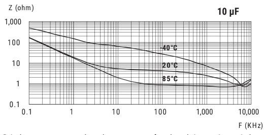
$R_{_{\rm e}}$  is the most temperature-dependent component of an electrolytic capacitor equivalent circuit. Electrolyte resistivity will decrease if temperature rises.
