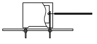
Temperature monitored inside the capacitor.
