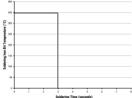
Soldering iron tip temperature should be set at 350°C (+10°C maximum), with the soldering duration not to exceed 3 seconds.
