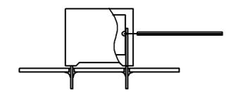
Temperature monitored inside the capacitor.
