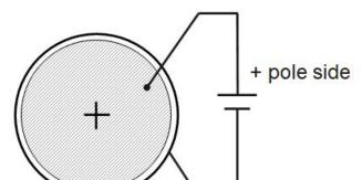
No sign is displayed on the – pole side of the polarization treatment.
