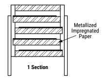
Film Capacitors – AC Line EMI Suppression and RC Networks PMR209, Metallized Impregnated Paper, Class X2, 250 VAC
