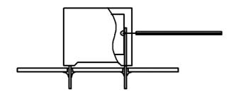
Temperature monitored inside the capacitor.
