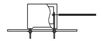
Temperature monitored inside the capacitor.
