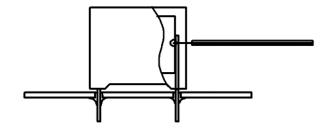
Temperature monitored inside the capacitor.
