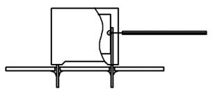
Temperature monitored inside the capacitor.
