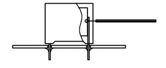
Temperature monitored inside the capacitor.
