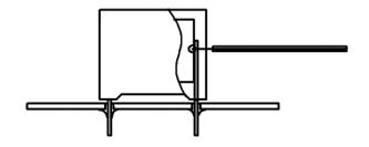
Temperature monitored inside the capacitor.
