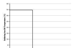
The soldering iron tip temperature should be set at 350°C (+10°C maximum) with the soldering duration not to exceed more than 3 seconds.
