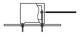
*Temperature monitored inside the capacitor.*
