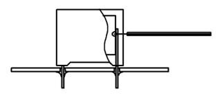
Temperature monitored inside the capacitor.
