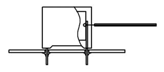
*Temperature monitored inside the capacitor.*
