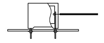
Temperature monitored inside the capacitor.
