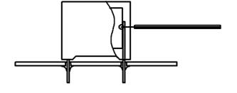
Temperature monitored inside the capacitor.
