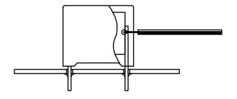
Temperature monitored inside the capacitor.
